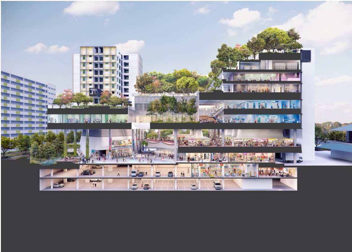
Kampung Admiralty HDB housing in Singapore. Section showing the 3D layering of housing, mix use (food court, retail), health, children and elder care amenities, and gardens in the sky with a terraced community farm. Architect: WOHA.
