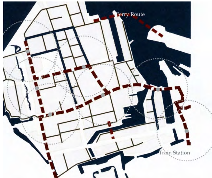
Public transport plan for Bo01. The plan ensures that no residence is more than 300 metres from a bus stop. Source: City of Malmö, 'Design Principles'. Redrawn by Mahammad Mornin.
