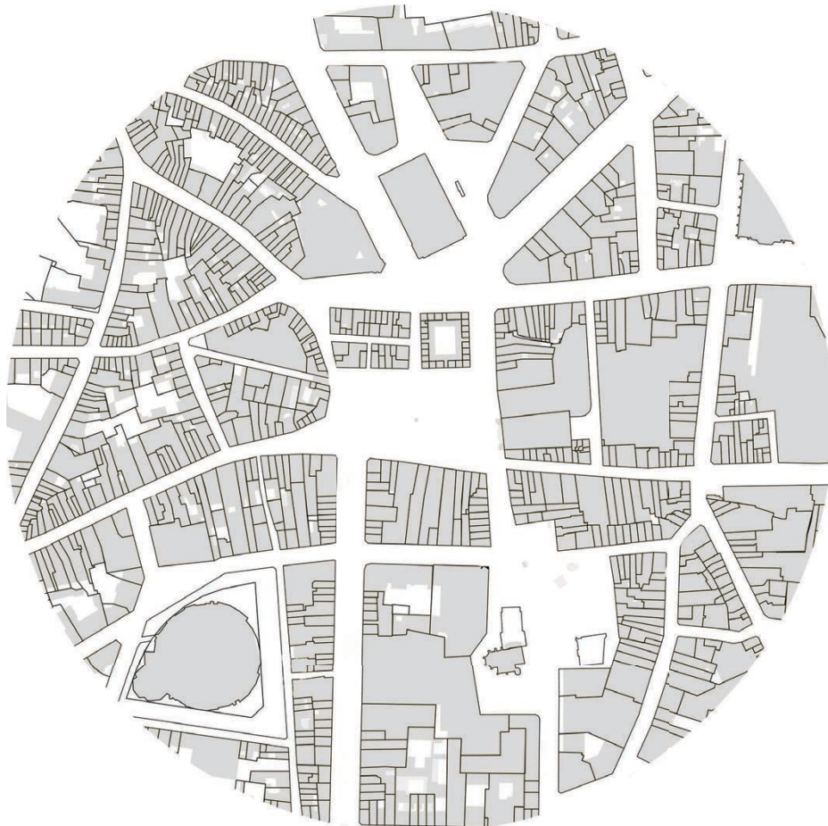
Plot pattern around Lille Grand place within a circle 300-m radius. Drawing by Emile Tack. École Spéciale d'Architecture, Paris.
