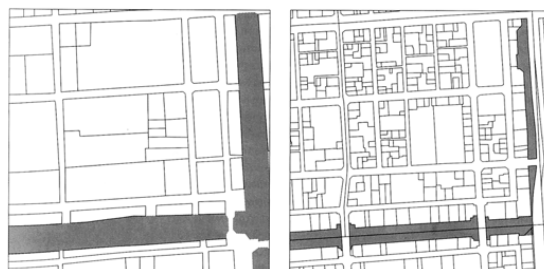
Unlike the American plot, the Japanese plot is subdivided and becomes more complex over time, creating a 'fractal' city where the land use testifies to a complex society. Comparison of plot structure between the mid 19th-century Edo period (left) and the same site at present (right). Source: Firley and Stahl 2009.
