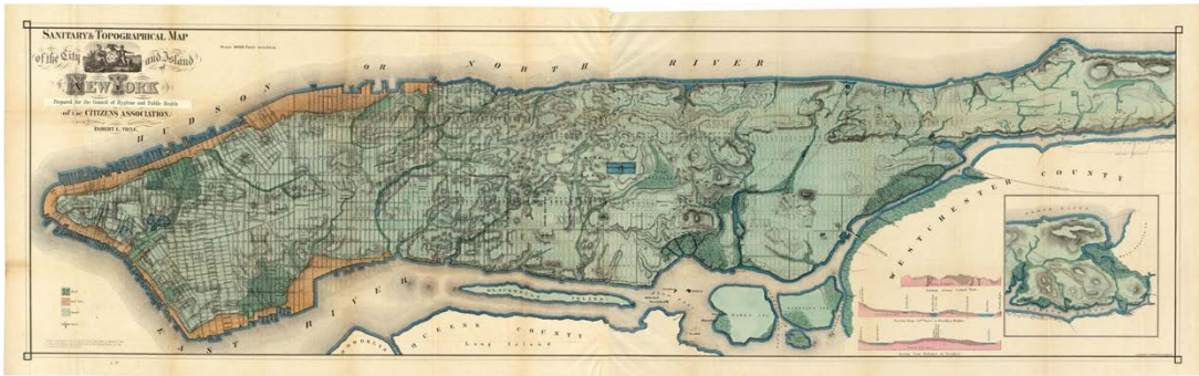
The Viele map. This map from 1865 by the civil engineer Egbert Ludovicus Viele shows not only the current grid but a pre-development view of Manhattan's topography and hydrology.
