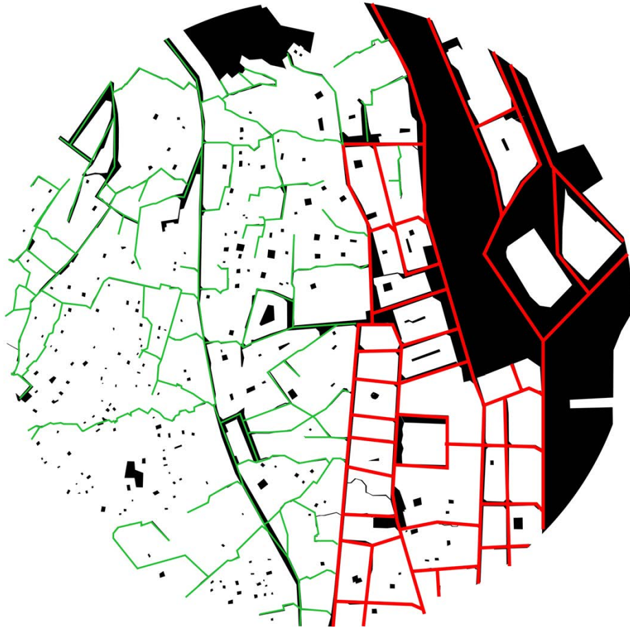
Casbah, Algiers. Drawings by Melissa Lyria Khali. École Spéciale d'Architecture, Paris. In red: Planned European grid. In green: Arabic organic pattern.
