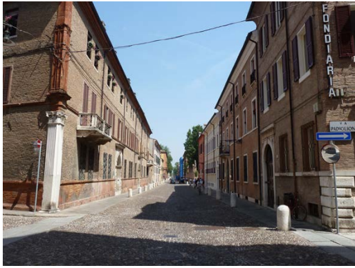
Ferrara. The reinforcement of block corners by white marble pilasters. Photos: © Françoise Labbé.
